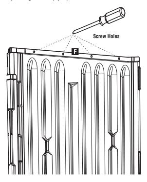
Connect Right Back (F) onto dovetails of Repeat Right Side (E).
